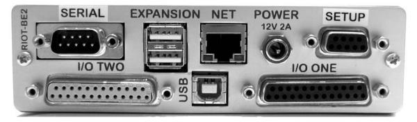
The back of each RIOT box has the following components:
